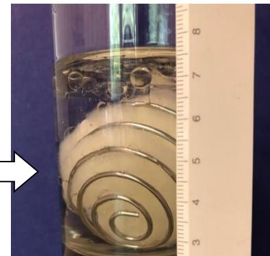
5. Start a timer when the sorbent has been submerged. Let it sit for 30 seconds, then lift it out (use tweezers) and let the filter drain back into the cylinder for an additional 30 seconds.
